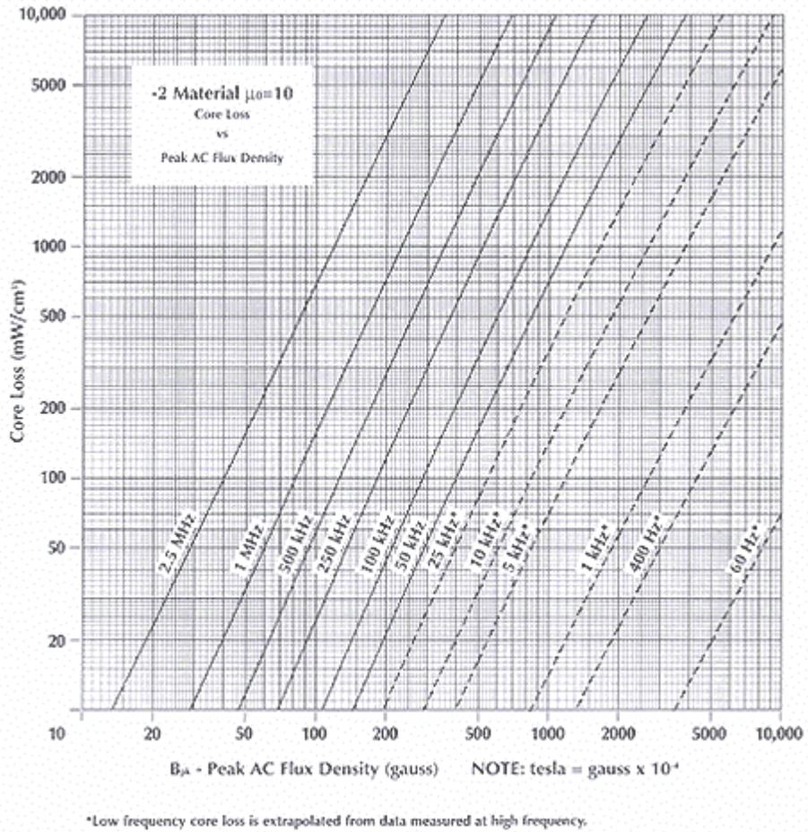
This data is for the fundamental only. To account for a square wave allow an extra 50%.
